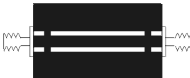
Figure 2 Printed Inductively Coupled Transmission Line Resonator
